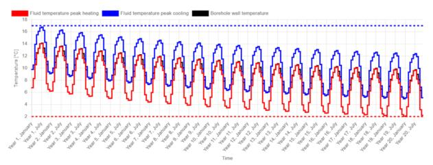
If we were to install additional geothermal power onto this borefield, we could exchange more energy with the ground, but we would not be able to extract more power during peak periods. This is why we say that this borefield has **potential for energy** but not for power, as the peak power already reaches the temperature limitations.
