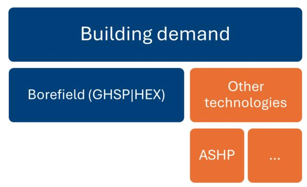
A hybrid geothermal system could be the solution. By adding other technologies—like an air source heat pump (ASHP)—to the borefield, you create a hybrid system where multiple technologies work together to provide heating and cooling. The combination of technologies
